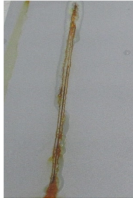
After 480 hours Salt Spray Test
