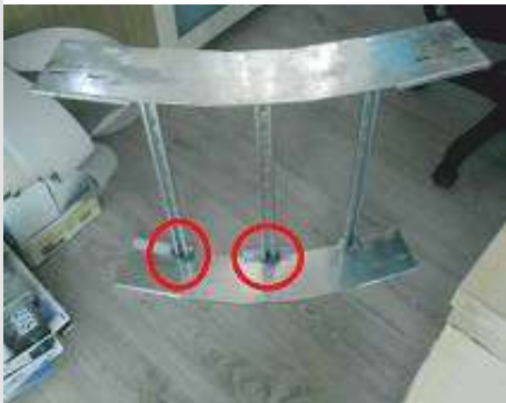
Uncoated areas in welding zone
